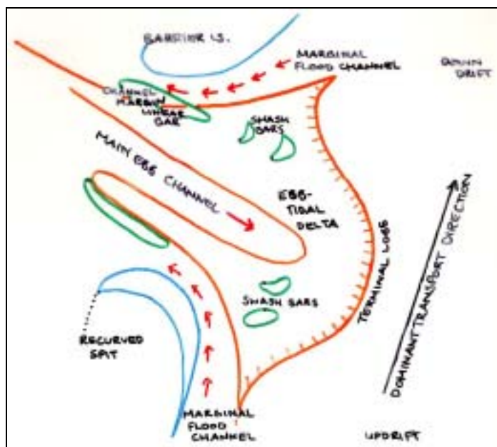
Figure A.2. Visual definition of the morphological components of a typical tidal inlet (Source: Adapted from Hayes, 1991)
