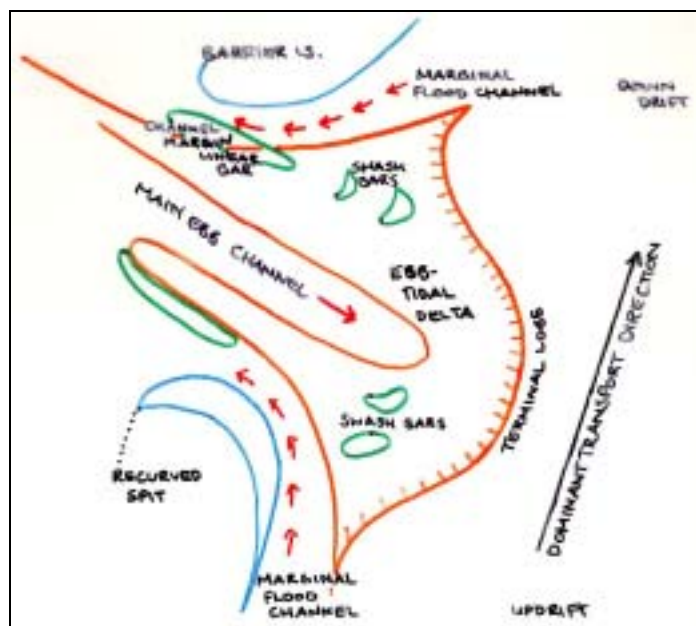
Figure 5.2. Typical ebb-tidal delta morphology (Source: Adapted from Hayes, 1991)
